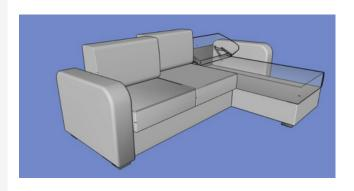
The lift is designed for installation in corner sofas. The lift allows you to change the angle of the backrest from a sitting position to a semi-reclining position with a 130-degree angle, creating a RELAX function.
